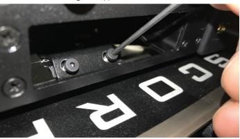
**STEP 9** Secure the SL-2 to the Scorpio with two 6 mm screws on either side of the Expansion Connector as shown in the image below using the supplied 2 mm Allen Wrench.
