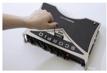
**STEP 4** Remove the safety mount from the top panel of Scorpio.
