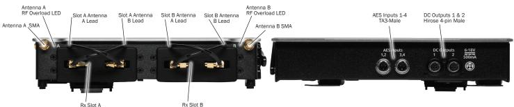
**ANTENNA A & B SMA CONNECTORS** Connects antenna to the SL-2. Both SMA antenna connectors can provide 12 V bias power up to 500 mA via a menu option. RF frequency range covers 470 - 1260 MHz. RF Filtering is available in the menus.
